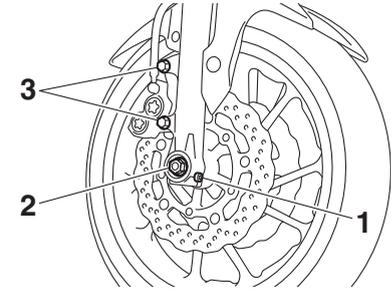
1. Front wheel axle pinch bolt
