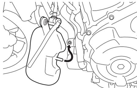
8. Remove the coolant drain bolt and its gasket to drain the coolant from the cooling system.
