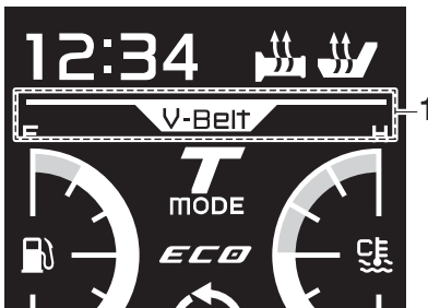
1. V-belt replacement indicator “V-Belt”
