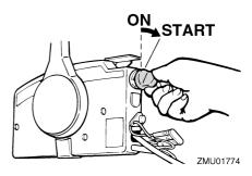
Immediately after the engine starts, release the main switch and allow it to return to "ON" (on).
