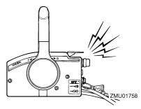
If the warning system has activated, stop the engine and check the cooling water inlet for clogging.
