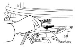
Press the power trim and tilt switch / power tilt switch "UP" (up) until the outboard motor has tilted up completely.
