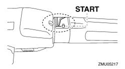
Turn the main switch to "START" (start), and hold it for a maximum of 5 seconds.
