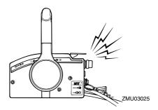
If the warning system has been activated, stop the engine and check for the cause.
