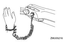
Place the throttle grip in the "START" (start) position. After the engine starts, return the throttle to the fully closed position.
