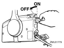
2. After stopping the engine, disconnect the fuel line if there is a fuel joint on the outboard motor.
