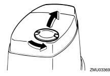
2. Open the oil tank filler cap by pulling the tab on the cap.
