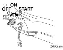
Immediately after the engine starts, release the main switch and allow it to return to "ON" (on).
