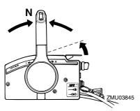
5. Turn the main switch to "ON" (on).
