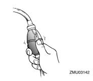
4. Open the throttle slightly without shifting using the throttle grip, neutral throttle lever or free accelerator. It is necessary to change the throttle opening slightly depending on the engine temperature. After the engine starts, return the throttle to its original position.
